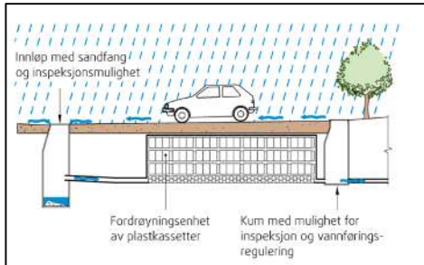
Prinsipp for plastkassetter
